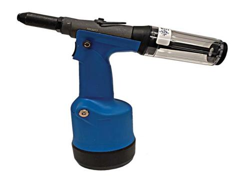
The HR-568 is a powerful and durable lightweight tool with surprising features found in many of our more expensive tools. For example, the tool comes with an adjustable mandrel collection system that holds rivets in the tool and allows rivets to be set even upside down. It has a long stroke which enables larger rivet diameters to be set in a single pull. Rated for 5,000 cycles before maintenance. The tool even comes with extra jaws, jaw springs & jaw housing.
